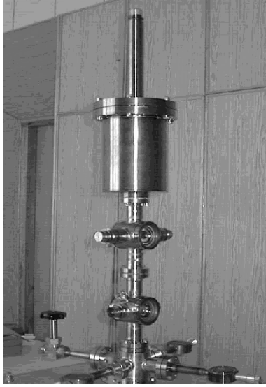
Fig.4. Vacuum part of CsFW (photo).
