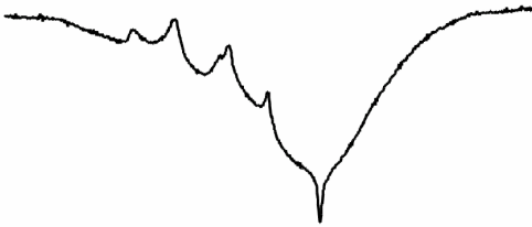
Fig.7. The saturated absorption signal with an inverted F=4-F'=5 pick used for the laser-frequency stabilization. The left pick corresponds to the principal line F=4-F'=3 transition, the right pick is the principal line of F=4-F'=5 transition. All cross-over picks in between.
